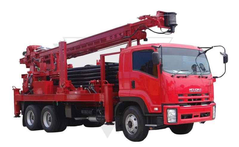
A robust deep hole drilling rig with a pull up force of 14100 kg capable of drilling 6 ½" diameters up to 450 m depth. Drilling hole size range from 6 ½" to 14".
